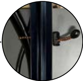
These bungee cords can be used to manage cables under the surface.
